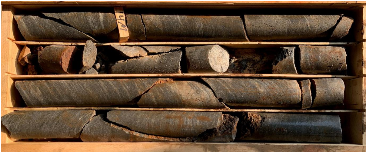
Figure 1: Hole CMD 23-017 Core with Graphite Mineralization with Approximately 3.4% Grade (Cg)
