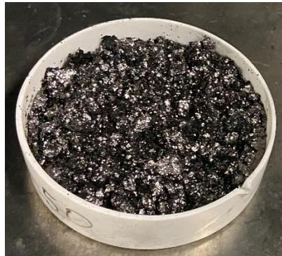
**Figure 3 – +50 Mesh Natural & Expanded Graphite**
